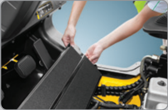
Tool-less floor plate for serviceability.
