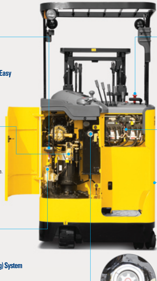
ORFS (O-Ring Face Seal) ORFS type hose prevents the leaking of hydraulic oil.
