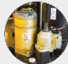
EPS (Electric Power Steering) System
