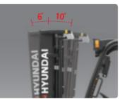
**Increased Mast Tilting Angle** Utilizing the mast tilting angle of 6 degrees forward and 10 degrees backward, the operator can safely and rapidly perform loading and unloading jobs.
