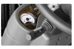
**Easy and Safe Shift Lever** A single lever on the left side of the steering column gives the operator fast, easy control of direction. The lever must be in the neutral position before the engine can be started.
