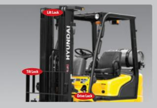
**OPSS (Operator Presence Sensing System)** Control of mast tilting, lifting and lowering is not possible through operation of the appropriate control when the not in the seated position.
