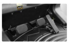
**Ergonomically Positioned Pedals** Based on human engineering, the accelerator, brake and inching pedals are optimally positioned for convenience while operating the equipment.
