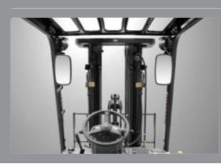
New High Visibility for Safe Operation The operator is able to work with increased safety and accuracy due to a wider view mast.
