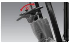
**Adjustable Steering Wheel** Steering wheel with horn button can be adjusted by a lever on the right-hand side for the most comfortable operator position.
