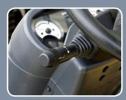
**Easy and safe shift lever** A single lever on the left side of the steering column gives the operator fast and easy controls of the direction.
