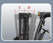
**Increased mast tilting angle** The mast tilting angle of 8 degrees forward and 10 degrees backward, the operator can safely and rapidly perform loading and unloading jobs.
