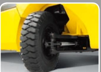
**Fully hydrostatic power steering**
